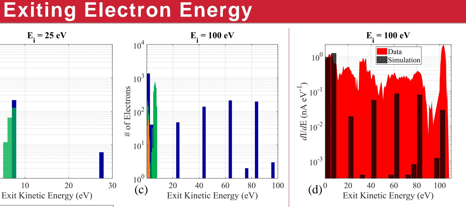
(d) Comparison between the experimental data obtained by analyzing the electron beam with a retarding field and the distribution of the electron energies obtained from the simulation. Again, these data were collected for  $n_{Rb} = 10^{13}$  cm<sup>-3</sup> and  $P_{N_2} =$ 130 *mTorr*.
