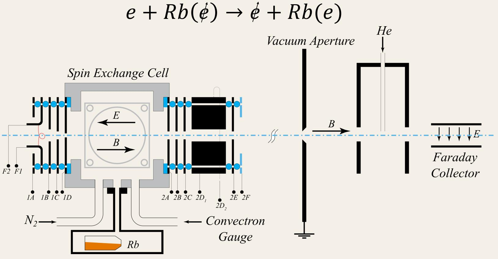
Thermionically emitted electrons from the filament (F1/F2) propagate through the Spin Exchange Cell, which contains N<sub>2</sub> and polarized Rb. The electron current passing through the cell picks up a net spin polarization, which is analyzed with a helium polarimeter and Faraday Collector.
