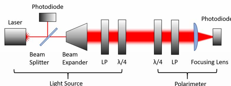
**Figure 2.** Polarimeter Setup. From left to right: laser, beam splitter and photodiode for drift normalization, beam expander to increase illuminated area of 2-inch polarization optics, polarization-state-defining linear polarizer (LP) and quarter waveplate ( $\lambda/4$ ), stepper-motor-controlled analyzing quarter waveplate and linear polarizer, focusing lens, and photodiode.
