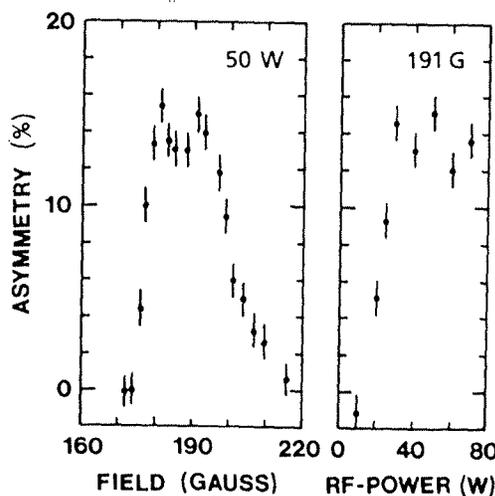
Fig.4. Tuning of the high frequency (1.49 GHz) rf transition region in the polarized  $H^0$ -stage of the source for maximum  $P^+$  polarization of the  $H^-$  beam. Correspondingly, there is a low-frequency (19.5 MHz) transition region for the  $P^+$  polarization.
