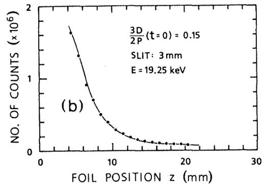
Fig.3. Measured circular polarization of Ly-α photons and intensity vs. foil position. The curves are fits to the functional forms given in Fig.2, with instrumental acceptance and resolution included, from which an average proton polarization of P=0.74 was deduced.
