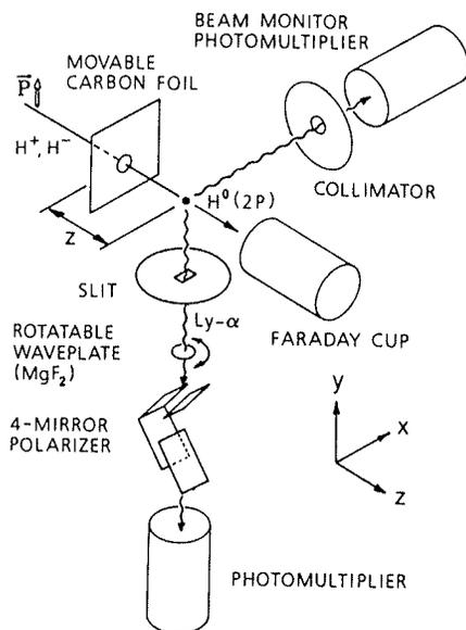
Fig. 1. Beam-Foil Proton Polarimeter
