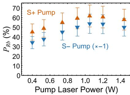
**FIG. 6.** Rubidium polarization  $P_{Rb}$  vs laser power for both helicities of pump light. We observe that the polarization saturates at  $\sim 1$  W of laser power. The data were collected with 330 mTorr of  $N_2$  buffer gas and a pump laser detuning of +1.5 GHz.
