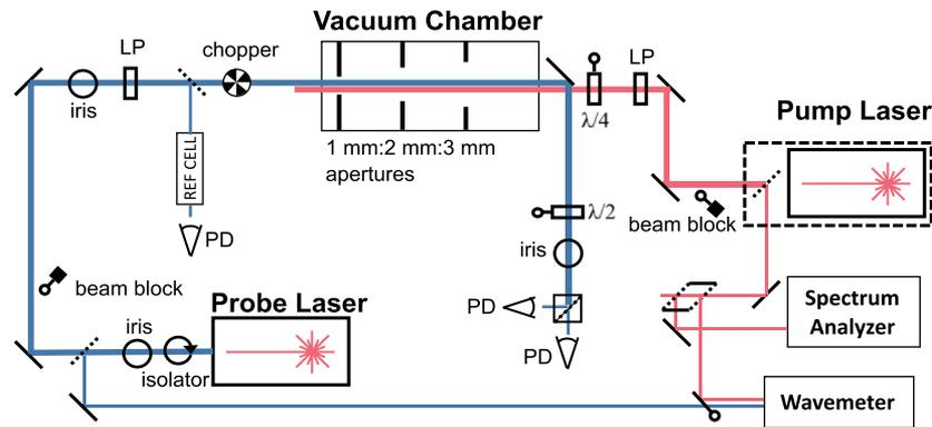
**FIG. 3.** A schematic of the optics used to optically pump Rb and to measure its density and polarization. The small circles connected to various optical elements indicate that they are computer controlled. LP = linear polarizer,  $\lambda/4$  = quarter-wave plate,  $\lambda/2$  = half-wave plate, and PD = photodiode.
