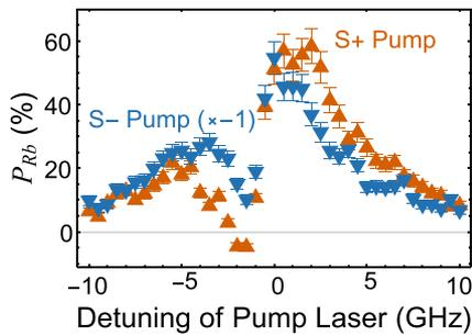
**FIG. 5.** The relationship between the pump laser frequency and rubidium polarization,  $P_{Rb}$ . The highest magnitude of polarization was obtained at 1.5 GHz with S+ pump light, so this was the frequency used to generate spin-polarized electrons. We observe the spin reversal phenomenon<sup>17</sup> at  $\sim -1.5$  GHz; the magnitude is smaller than that has been observed previously, indicating that we have purer circular light polarization.
