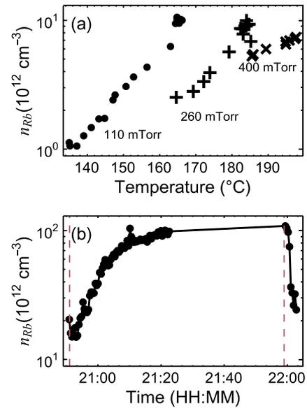
**FIG. 7.** (a) The interaction between  $\mathcal{P}_{BG}$  and  $n_{Rb}$  as the reservoir temperature is varied. (b) Rb density in the spin-exchange cell vs time as  $\mathcal{P}_{BG}$  is adjusted. The vertical dashed lines indicate when  $\mathcal{P}_{BG}$  is changed; the line on the left corresponds to an abrupt drop from 400 to 130 mTorr, while the one on the right indicates an increase back up to 400 mTorr. The solid line is drawn to guide the eye.
