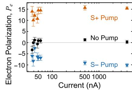
**FIG. 11.** Electron polarization,  $P_e$ , as a function of output current. These data were collected with 400 mTorr of  $N_2$  at an electron beam energy of 140 eV.
