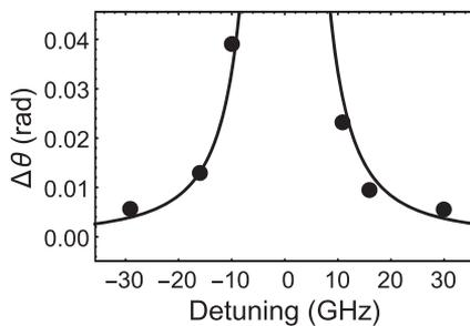
**FIG. 4.** Typical data collected to measure the Rb number density. As the detuning approaches zero, the polarization angle of the probe laser ( $\theta$ ) shifts. Angles are measured at six detuning frequencies (data points) and fit to Eq. (1) (solid line). The calculated number density for this dataset is  $3.7(7) \times 10^{12} \text{ cm}^{-3}$ .
