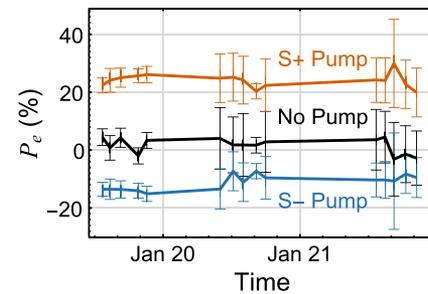
**FIG. 17.** Electron polarization  $P_e$  taken over the course of several days; these data were collected with  $E_i = 100$  eV,  $\mathcal{P}_{BG} = 400$  mTorr  $N_2$ , and  $n_{Rb} = 5 \times 10^{12}$  cm<sup>-3</sup>. The current of the electron beam was  $\sim 300$  nA.
