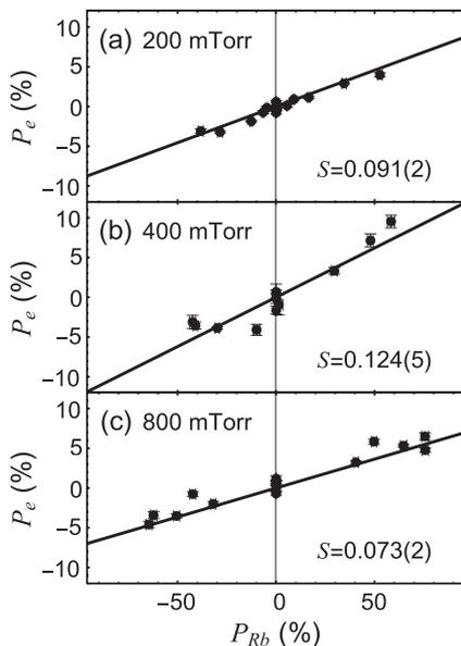
**FIG. 13.** (a)–(c) A measurement of the spin transfer efficiency  $S$  for  $N_2$  buffer gas pressures of 200, 400, and 800 mTorr. The electron polarization  $P_e$  vs  $P_{Rb}$  with  $n_{Rb} = 10 \times 10^{12} \text{ cm}^{-3}$  is plotted as the pump laser is tuned off resonance to vary  $P_{Rb}$ . The slope of a linear fit fixed through the origin gives the value of  $S$ . For each of these runs, the energy of the electrons incident on the Rb,  $E_i$ , was 100 eV.
