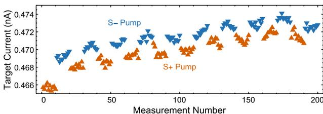
**FIG. 19.** Preliminary raw data searching for an asymmetry in secondary electron emission from cysteine. Although the data appear to have a large asymmetry, a significant portion of this is instrumental in nature. This figure simply illustrates the signal we analyze. The upward-pointing and downward-pointing symbols correspond to the two different helicities of the polarized electron beam.
