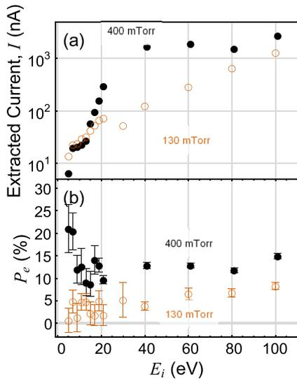
**FIG. 18.** The filled circles show the present performance of the apparatus, while the open circles, collected recently at  $\mathcal{P}_{BG} = 130$  mTorr, approximate the previous performance of the apparatus.<sup>10</sup> (a) Operating the system at  $\mathcal{P}_{BG} = 400$  mTorr resulted in improved values of  $P_e$  for all values of  $E_i$ . (b) The transmitted current was improved for intermediate energies but was slightly reduced for low and high values of  $E_i$ .
