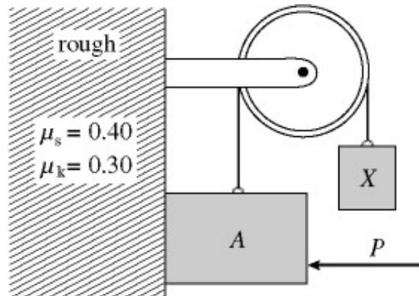
Block A of mass 8 kg and block X are attached to a rope that passes over a pulley. A 50 N force  $P$  is applied horizontally to block A, keeping it in contact with a rough vertical face. The coefficients of static and kinetic friction between the wall and block A are  $\mu_s = 0.4$ ,  $\mu_k = 0.3$ . The pulley is light and frictionless. Determine the mass of block X such that block A descends at a constant velocity of 5 cm/s when it is set into motion.
