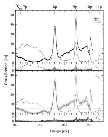
**Figure 10.** Data equivalent to that in figure 5 except for reaction (6): 514.5 nm—Ar<sup>+</sup>  $3p^4$  [<sup>3</sup>P] 4p (<sup>4</sup>D<sub>5/2</sub>) to  $3p^4$  [<sup>3</sup>P] 4s (<sup>2</sup>P<sub>3/2</sub>). The experimental resolution and the convolution width of the theoretical calculation are 5 meV.
