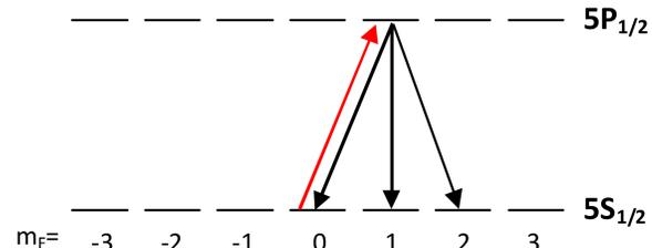
**Typical Optical Pumping** for an  $F=3$  state using D1 light (with  $^{85}\text{Rb}$ ,  $I=5/2$ ). The red arrow represents the absorption of a circularly-polarized photon and the black arrows represent the available decay channels. In this situation, atoms that are pumped to the  $m_F=3$  state become dark and are said to be completely polarized.
