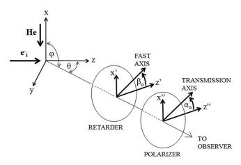
FIG. 1. Schematic of the He optical electron polarimeter geometry. In our device,  $\varphi=90^\circ$  and  $\theta=36.5^\circ$ . The electron beam is incident along z while the helium gas flows towards the -x direction. The initial offsets of the retarder's fast axis and the linear polarizer's transmission axis are denoted by  $\beta_o$  and  $\alpha_o$ , respectively.
