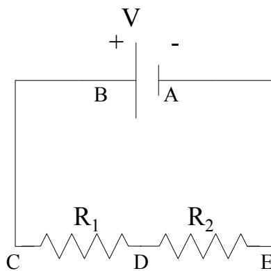
Consider a circuit consisting of two resistors,  $R_1$  and  $R_2$  and a battery with a voltage  $V$ .
