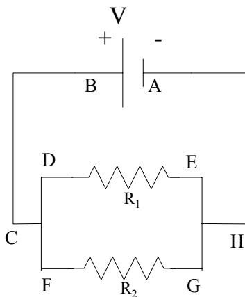
In some cases, we want to hook up electrical resistances in parallel, as shown to the left. Let the battery again have voltage  $V$ .
