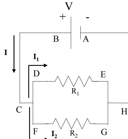
$$I_1 = \frac{V}{R_1} \quad I_2 = \frac{V}{R_2}$$
