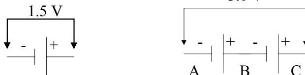
potential at point A is 0 V, at point B is 1.5 V and at point C is 3.0 V.
