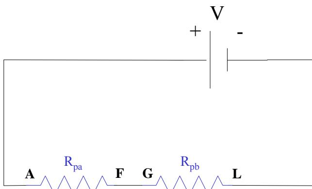
$$\frac{1}{R_{pb}} = \frac{1}{R_3} + \frac{1}{R_4} + \frac{1}{R_5}$$
