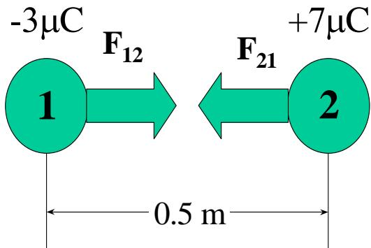
The negative sign means that the forces are attractive. If we draw the picture as shown at left, the force that 1 exerts on 2 ( $F_{21}$ ) is to the left. The force that 2 exerts on 1 ( $F_{12}$ ) is of the same magnitude and to the right.
