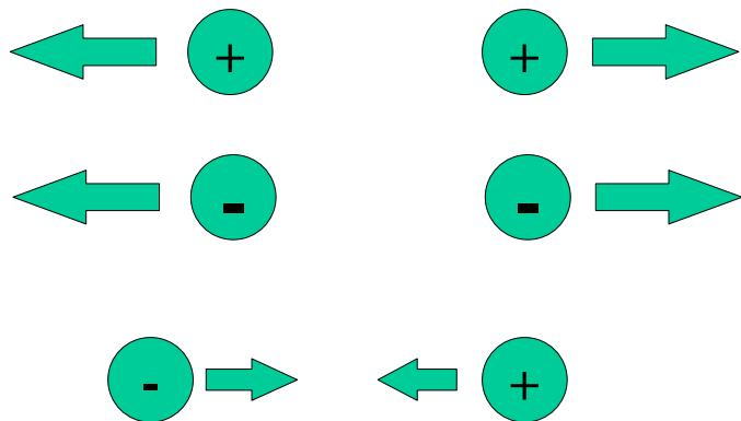
If  $q_1 > 0$  and  $q_2 > 0$ , then  $F$  will be positive. This corresponds to the two charges trying to repel each other. Note that the force the two charges exert will be equal and opposite in all cases. The same situation applies when the two charges are both positive. When the sign on the force is positive, the force is **repulsive**.
