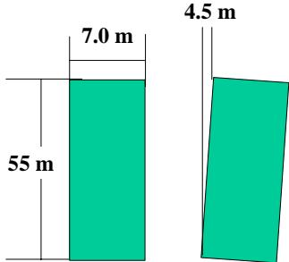
The center of gravity will be located at the middle of the tower – we're treating it as if it were uniform.
