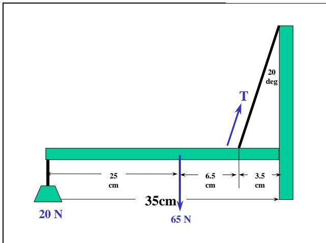
We can model the arm as shown. Note that the CM (center of mass) is NOT at the geometric center of the object: this is because the mass is not uniformly distributed along the arm. The location of the CM would have to be given to you for you to work the problem.
