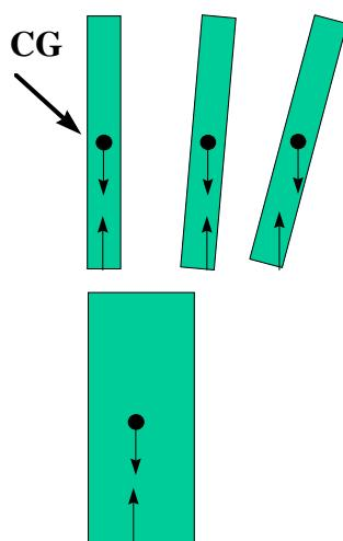
As soon as the ruler's CG is no longer over the base, the force of gravity causes an unbalanced torque and the ruler will fall. The eraser has a much broader base, and therefore can be tipped further before the cg extends over the base.
