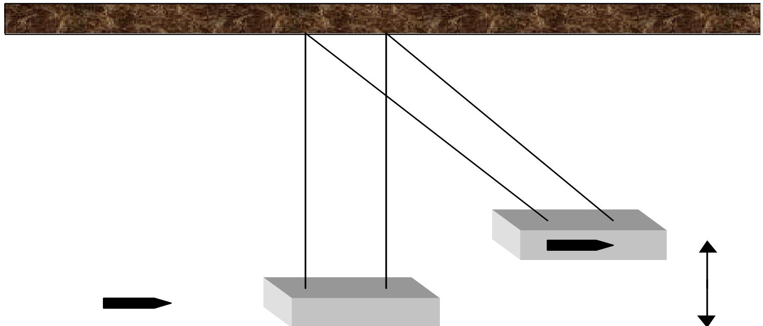
We can apply conservation of momentum during the collision (bullet to block). The momentum before the bullet hits must be equal to the momentum after the bullet hits.
