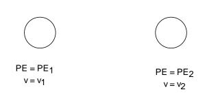
and has potential energy  $PE_1$ . At some later time, the object now has velocity  $v_2$  and potential energy  $PE_2$ . In order to make the change from the first situation to the second, work must be done on the object. That work can be divided into two parts: a part due to conservative forces,  $W_C$  and a part due to nonconservative forces  $W_{NC}$ .
