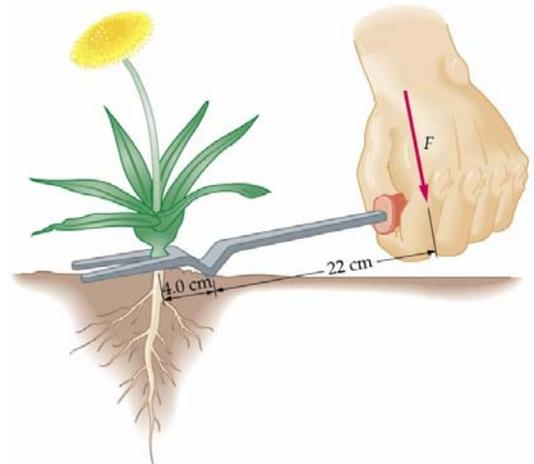
Note that we are assuming that static equilibrium prevails. The force the gardener exerts on the tool and the force the weed exerts on the tool cause equal and opposite torques about the pivot. Thus, if the gardener pulled just a little bit harder the weed would come out.
