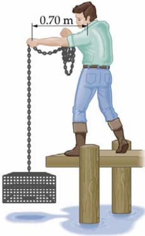
To counteract the torque created by the weight of the trap (and neglecting the weight of the arm and rope), the torque exerted about the shoulder must be
