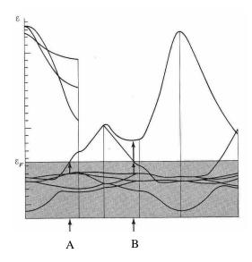
**Fig.5** Calculated bands for copper, illustrating that the absorption threshold for transitions up from the conduction band is about 4 eV, while the threshold for transitions from the d-band to the conduction band is only about 2 eV. The energy scale is in tenths of a rydberg (0.1 Ry = 1.36 eV).
