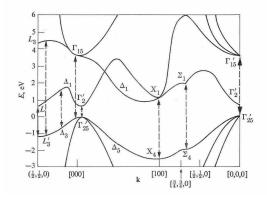
**Fig. 7** (a) Imaginary dielectric constant versus photon energy for Ge. (b) The band structure of Ge. Dashed arrows indicate various critical points. [After Phillips, 1966]
