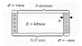
Fig. 2 Simple model of a plasma oscillation.
