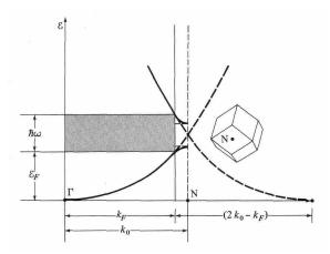
**Fig.4.** Free electron determination of the threshold energy for interband absorption in the alkali metals. Numerically,  $\hbar\omega = 0.64E_F$ .
