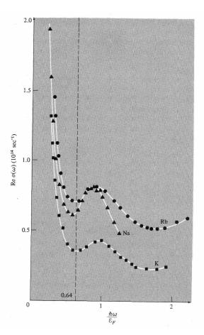
**Fig.3.** Re $\sigma(\omega)$ , deduced from reflectivity measurements in three alkali metals. The interband threshold is evident, and occurs quite close to  $0.64E_F$ , where  $E_F$  is the free electron Fermi energy.
