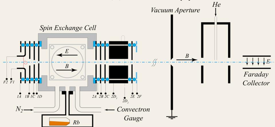
Thermionically emitted electrons from the filament (F1/F2) propagate through the Spin Exchange Cell, which contains  $N_2$  and polarized Rb. The electron current passing through the cell picks up a net spin polarization, which is analyzed with a helium polarimeter and Faraday Collector.
