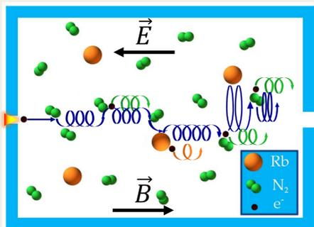
Illustration of electron propagation through the Spin Exchange Cell. Typical values:  $E = 100 \text{ V/m}$ ,  $B = 270 \text{ G}$ .
