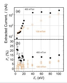
**FIG. 18.** The filled circles show the present performance of the apparatus, while the open circles, collected recently at  $\mathcal{P}_{BG}=130$  mTorr, approximate the previous performance of the apparatus. <sup>10</sup> (a) Operating the system at  $\mathcal{P}_{BG}=400$  mTorr resulted in improved values of  $P_e$  for all values of  $E_i$ . (b) The transmitted current was improved for intermediate energies but was slightly reduced for low and high values of  $E_i$ .
