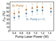
**FIG. 6.** Rubidium polarization  $P_{Rb}$  vs laser power for both helicities of pump light. We observe that the polarization saturates at ~1 W of laser power. The data were collected with 330 mTorr of  $N_2$  buffer gas and a pump laser detuning of +1.5 GHz.
