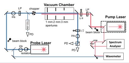
**FIG. 3.** A schematic of the optics used to optically pump Rb and to measure its density and polarization. The small circles connected to various optical elements indicate that they are computer controlled. LP = linear polarizer,  $\lambda/4$  = quarter-wave plate,  $\lambda/2$  = half-wave plate, and PD = photodiode.
