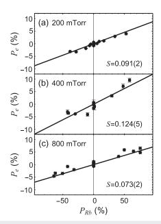
**FIG. 13.** (a)–(c) A measurement of the spin transfer efficiency S for  $N_2$  buffer gas pressures of 200, 400, and 800 mTorr. The electron polarization  $P_e$  vs  $P_{Rb}$  with  $n_{Rb} = 10 \times 10^{12}$  cm<sup>-3</sup> is plotted as the pump laser is tuned off resonance to vary  $P_{Rb}$ . The slope of a linear fit fixed through the origin gives the value of S. For each of these runs, the energy of the electrons incident on the Rb,  $E_i$ , was 100 eV.
