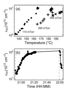
**FIG. 7.** (a) The interaction between  $\mathcal{P}_{BG}$  and  $n_{Rb}$  as the reservoir temperature is varied. (b) Rb density in the spin-exchange cell vs time as  $\mathcal{P}_{BG}$  is adjusted. The vertical dashed lines indicate when  $\mathcal{P}_{BG}$  is changed; the line on the left corresponds to an abrupt drop from 400 to 130 mTorr, while the one on the right indicates an increase back up to 400 mTorr. The solid line is drawn to guide the eye.
