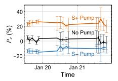
**FIG. 17.** Electron polarization  $P_e$  taken over the course of several days; these data were collected with  $E_i = 100$  eV,  $\mathcal{P}_{BG} = 400$  mTorr  $N_2$ , and  $n_{Rb} = 5 \times 10^{12}$  cm<sup>-3</sup>. The current of the electron beam was ~300 nA.
