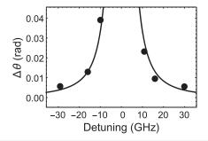
**FIG. 4.** Typical data collected to measure the Rb number density. As the detuning approaches zero, the polarization angle of the probe laser  $(\theta)$  shifts. Angles are measured at six detuning frequencies (data points) and fit to Eq. (1) (solid line). The calculated number density for this dataset is  $3.7(7) \times 10^{12} \text{ cm}^{-3}$ .
