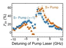
**FIG. 5.** The relationship between the pump laser frequency and rubidium polarization,  $P_{Rb}$ . The highest magnitude of polarization was obtained at 1.5 GHz with S+ pump light, so this was the frequency used to generate spin-polarized electrons. We observe the spin reversal phenomenon<sup>17</sup> at  $\sim$  –1.5 GHz; the magnitude is smaller than that has been observed previously, indicating that we have purer circular light polarization.
